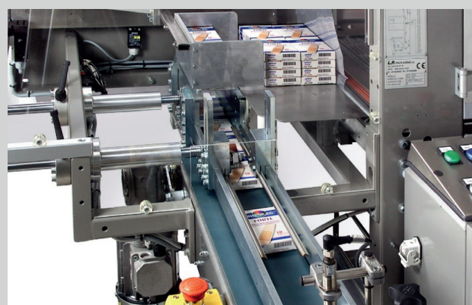
90° feeding with stacker device
