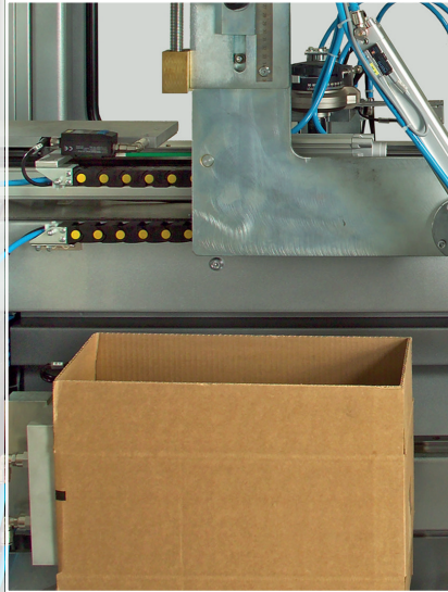
Forming box station with corrugated cardboard.
