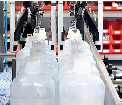
PICK AND PLACE FOR PRODUCTS WITH SCREW CAPS
